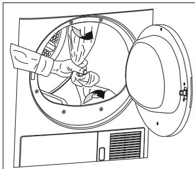
**⚠** Make sure that you have removed the transportation safety assembly (nylon+styrofoam pieces) before using the
