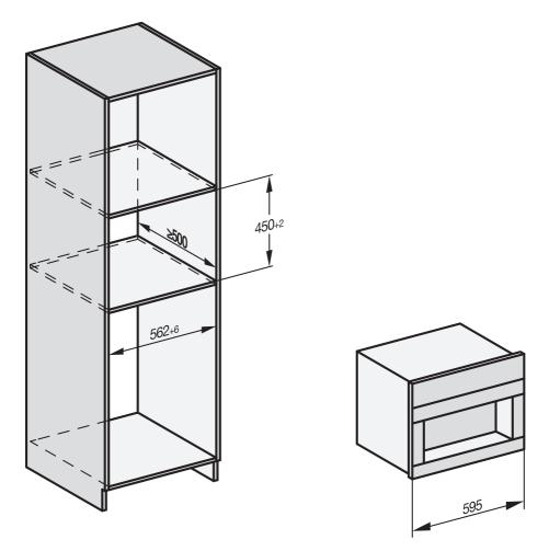
The machine can be combined with other Miele built-in appliances. In this case, there must be a full-width, closed shelf between them. If the machine it to be combined with a suitable built-in plate/food-warming drawer, no shelf is required in between.
