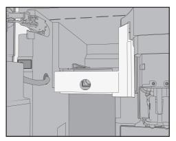
Remove the milk valve cover as follows: on the top right-hand side of the cover, you will find a pin for swivelling the cover out.
