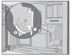
Press the button under the handle of the brew unit ① and, whilst doing so, turn the handle forwards ②.
