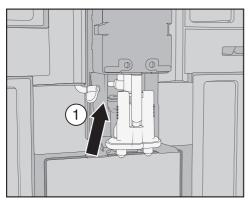
Detach the milk pipe from the dispensing unit as follows: pull the tab ① to the left.
