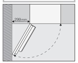
Check that there is a gap of at least 299 mm between the wall (or similar) and the coffee machine so that you can open the door wide enough to remove the left-hand bean container (minimum door opening angle of 120°).
