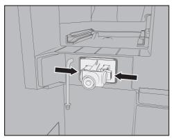
Press the retainers on the left and right-hand sides of the milk valve holder and pull the holder forwards to remove it.
