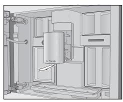
Pull the central spout's stainless steel cover forwards to remove it. Then clean it.
