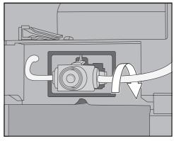
**Tip:** If necessary, screw the milk pipework backwards at the connecting piece on the right-hand side.
