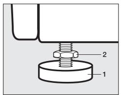
Using the spanner supplied turn counter nut 2 in a clockwise direction. Then unscrew counter nut 2 together with foot 1.
