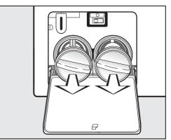
Remove the drain filters completely.
