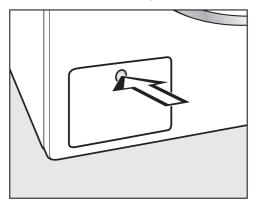
Press the drain pump access panel.
