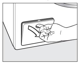
Open the drain pump access panel.
