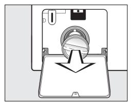
Remove the drain filter completely.
