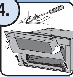
Push out retaining clip, remove appliance door
