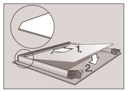
Then refit the middle glass pane together with the profiled seal.
