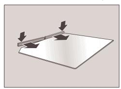
Secure the profiled seal to the middle glass pane.
