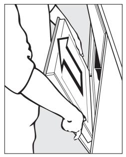
Hold the door on either side and pull it diagonally upwards off the retainers. Make sure that the door goes back on straight.
