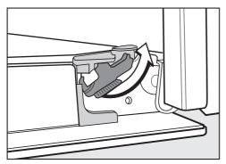
Release the locking clamps by turning them as far as they will go. The oven could become damaged if you incorrectly remove the door. Never pull the door horizontally off its retainers, as they will spring back against the oven.
