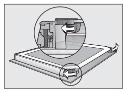
Flip the two glass pane retainers outwards to open them. Remove the inner pane:
