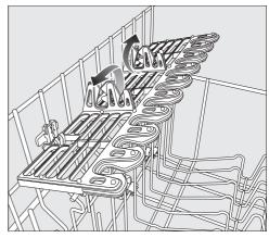
■ Fold up the MultiClips.
