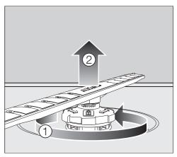
■ Rotate the screw thread of the lower spray arm anti-clockwise ① and pull the spray arm upwards to remove ②.
