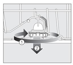
■ Rotate the screw thread of the middle spray arm clockwise ① (see diagram) and remove the spray arm ②.
