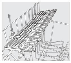
■ Slide the glass rack to the desired height until the catches click into place at the top or the bottom.
