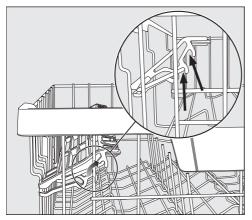
Pull the cup rack upwards and click it into the desired position (see arrow).
