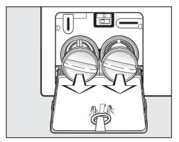
■ Remove the filters completely.
