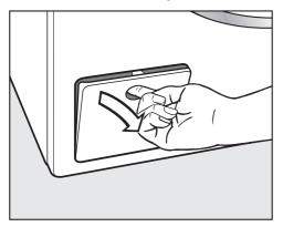
■ Open the drain pump access panel.
