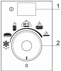
1 ON/OFF switch Turns the appliance on and off. 2 Temperature knob
