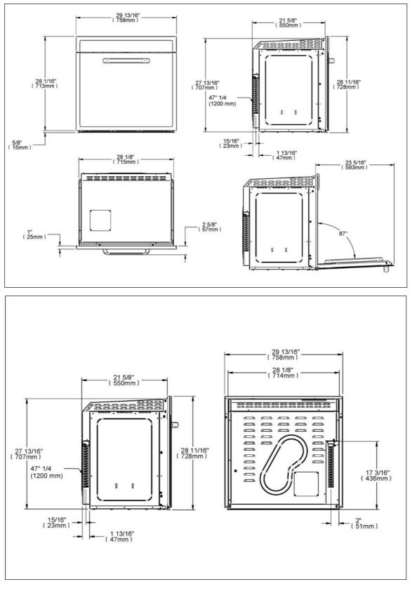
Electrical requirements 120/240V - 5500W (24 A max) or 120/208V - 4400W (21 A max). Upper heating element 3400W Lower heating element 2100W Convection heating elements 2 x 1650W
