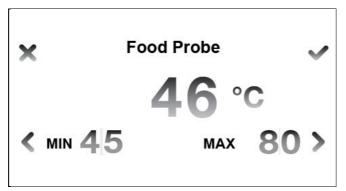
When using the food probe, the display will show the food probe temperature (actual and target) instead of the remaining time until the end of cooking.
