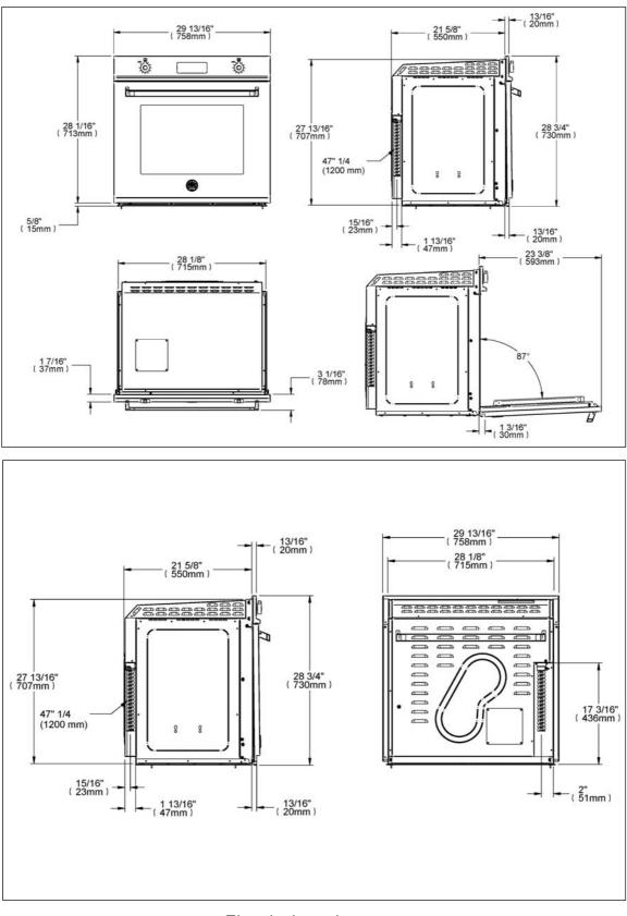
Electrical requirements 120/240V - 5500W (24 A max) or 120/208V - 4400W (21 A max). Upper heating element 3400W Lower heating element 2100W Convection heating elements 2 x 1650W
