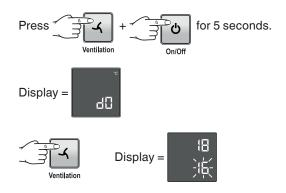
The refrigeration unit switches on. The temperature display flashes.
