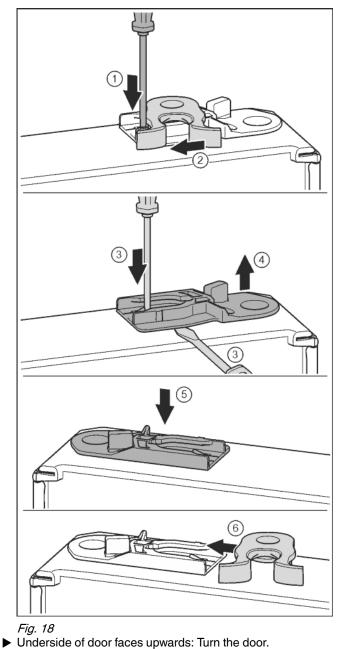
Push the lug downwards with a slotted screwdriver.
