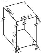
Then support the door: Use saddle wrench SW10 to unscrew the base on mounting block (B) until it makes contact with the ground, then continue turning it for a further 90°.
