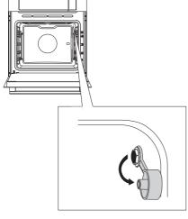
Remove the cap (the socket is in the front upper corner of the oven right wall).
