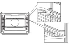
The grid or the tray should always be inserted into the groove between the two wire profiles.
