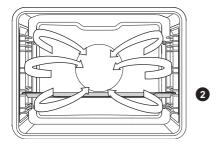
Water from the steam generator enters the oven cavity in the form of steam. In addition, round heater with fan operates to provide continuous circulation of the hot air and steam.
