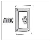
**?** Remove the halogen bulb.
