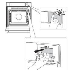
Press (on the spot with the sticker) to open the tank door.
