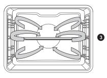
Round heater and the fan will operate. The fan installed on the back wall of the oven cavity makes sure the hot air constantly circulates around the meat, vegetables, or pastry.
