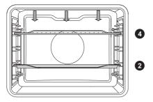
When grilling food with the large grill, the upper heater and the grill heater fitted on the ceiling of the oven cavity will operate.
