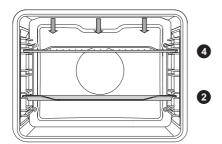
When grilling food with the large grill, the upper heater and the grill heater fitted on the ceiling of the oven cavity will operate.
