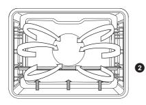
This is used for baking leavened but lowrising pastry and for preserving fruit and vegetables. Use the second guide from the bottom and a rather shallow baking tray to allow the hot air to circulate across the upper side of the dish.
