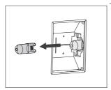
2 Remove the halogen bulb.
