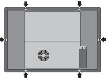
To install the clips into the hob, all you have to do is insert them horizontally into the appropriate space by applying light pressure.
