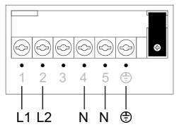
The adjacent diagram illustrates the power supply terminal from below, with no cables connected. Terminals 4 and 5 must be connected at all times.
