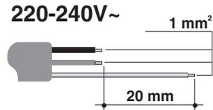
Use a **3 x 1 mm<sup>2</sup> three-core** cable.
