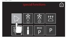
2. Enter the required duration (for example 25 minutes: first touch the minutes box. then the numbers 2 and 5).
