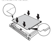
7. Reposition the internal glass pane. Insert the front part into the relative seats (1). Then lower the rear part and insert the 2 pins into their housings in the oven door by applying slight pressure (2).
