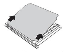
Some models have an intermediate glass unit. Remove the intermediate glass unit by lifting it upwards.
