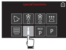
2. Press the symbol to start the Sabbath function, or press the preset temperature value to change it (from 60° to 100° C).
