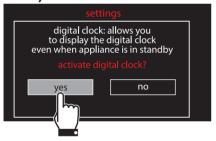
When no appliance function is active, the display will show the current time in digital format.
