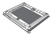
6. Refit the panes in the reverse order in which they were removed. Make sure that the upper shaped part of the intermediate glass unit is facing upwards towards the handle.
