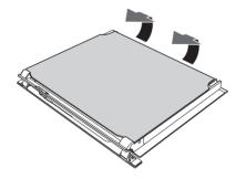
3. Then pull the front part upwards. This way, the 4 pins attached to the glass detach from their housings in the oven door.
