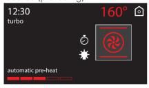
4. When the preheating stage is over a buzzer will sound to indicate that the food can be placed inside the oven.
