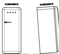
A few days after installation, check that the initial level adjustment is still correct. Make sure that the appliance is still stable and the door seals still close hermetically when it is in operation and loaded with food. If necessary, re-adjust the level and the seals.
