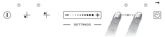
To change the power level (from 1 to max. 9 or P) press the -/+ buttons or slide your finger horizontally on the slider. To deactivate the Multizone function, press simultaneously the 2 selecting buttons of the zones. To switch off the zones instantly, hold one of the zone selection button for 3 seconds.
