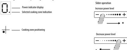
After switching the hob on, activate the required cooking zone by pressing the corresponding circular button and place the pot on the zone. With the Slider control it is possible to select the required power level, from min. 0 to max. 9, or booster "P" if available.
