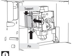
**N.B.:** If the brewing unit is difficult to insert, you must first adapt it to the right dimensions by pressing it forcefully from the bottom and top as shown in the figure.
