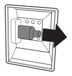
Do not touch the halogen lamp directly with your fingers, but hold it using insulating material.
