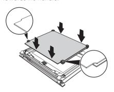
7. Reposition the internal glass panel. Insert the front part into the relative seats (1). Then lower the rear part and insert the 2 pins into their housings in the oven door by applying slight pressure (2).
