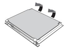
3. Then pull the front part of the glass panel upwards. In this way, the 4 pins attached to the glass detach from their housings in the oven door.
