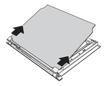
Some models are fitted with an intermediate glass unit. Remove the intermediate glass unit by lifting it upwards.
