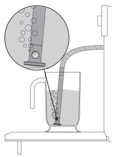
9. Press the **START** button to start filling the reservoir with water.
