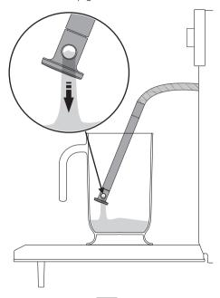
6. Press the START button to start draining the water into the jug.
