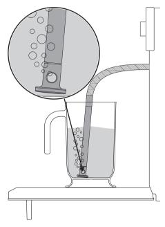
8. Touch the START button to start filling the reservoir with the descaler solution.
