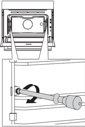
**1** Undo the screw. Use a screwdriver.
