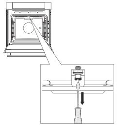
**1** To remove the heater, undo the screw located at the front of the oven cavity ceiling.
