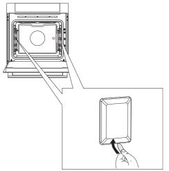
1 Use a flat screwdriver to release the bulb cover and remove it.
