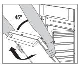
3 Slowly close the door to 2 angle (relative to the position of the Slowly close the door to a 45-degree fully closed door); then, lift the door and pull it out
