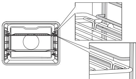
The grid or the tray should always be inserted into the groove between the two wire profiles.
