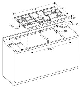
\* 61 mm in the area of the gas connection at the back right
