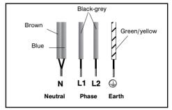
With hook-up of 400 V 2N three phase, verify that the neutral wire is properly connected.
