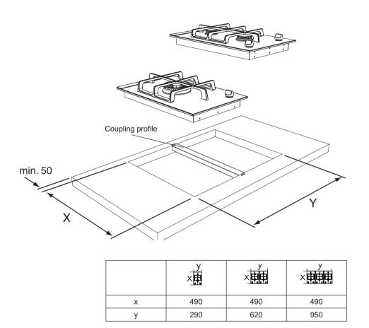
Use the coupling profiles provided when the units are fitted tightly together. Keep an edge of minimum 60 cm between the holes if the coupler is not used.
