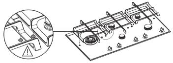
Assemble the burner parts with the aid of the guide ridges, paying attention to the cut-out sections in the burner head for the sparkplug and thermocouple. Make sure that the burner parts lie flat.
