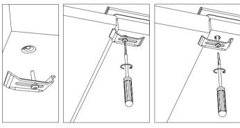
Screw hole Thin worktops for mounting bracket
