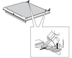
I Slightly lift the supports on the left and right side of the door (marking 1 on the support) and pull them away from the glass pane (marking 2 on the support).
