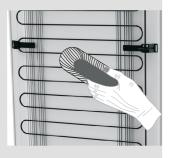
The condenser unit mounted on the (exterior) back wall should always be kept clean, free of dust or deposits resulting from kitchen smoke or fumes. Occasionally clean the dust using a soft non-metal brush or a vacuum cleaner.
