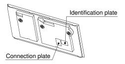
Affix the second identification plate (supplied) in an accessible position behind the front of the fitted cabinet beneath the appliance.
