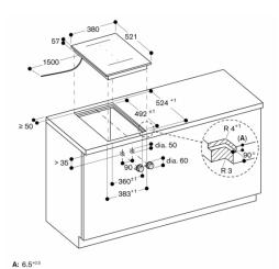
measurements in mm
