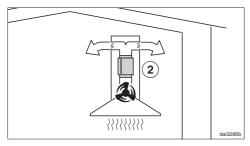
The silencer needs to be positioned between the exhaust connection and the directional unit (2). Ensure there is adequate space in the tower for fitting it.
