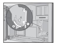
Press the button under the handle of the brew unit (1) and, whilst doing so, turn the handle forwards 1.
