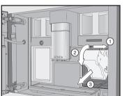
■ First, pull the brew unit sideways ① and then slide it out forwards 2. Tilt the
