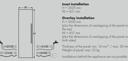
\* If a five-piece shaker style panel is used, which is thinner than the minimum panel thickness, shorter screws than those supplied in the accessory pack must be used.
