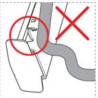
Incorrectly inserted trays or wire shelves may fall out of the runner!
