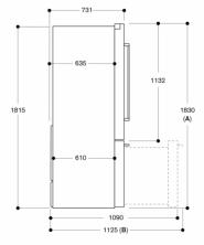
A: Front is adjustable from 1830 to 1847, with front levelling feet fully extended B: With handle measurements in mm
