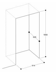
If you install the appliance in a niche, adhere to the dimensions shown measurements in mm
